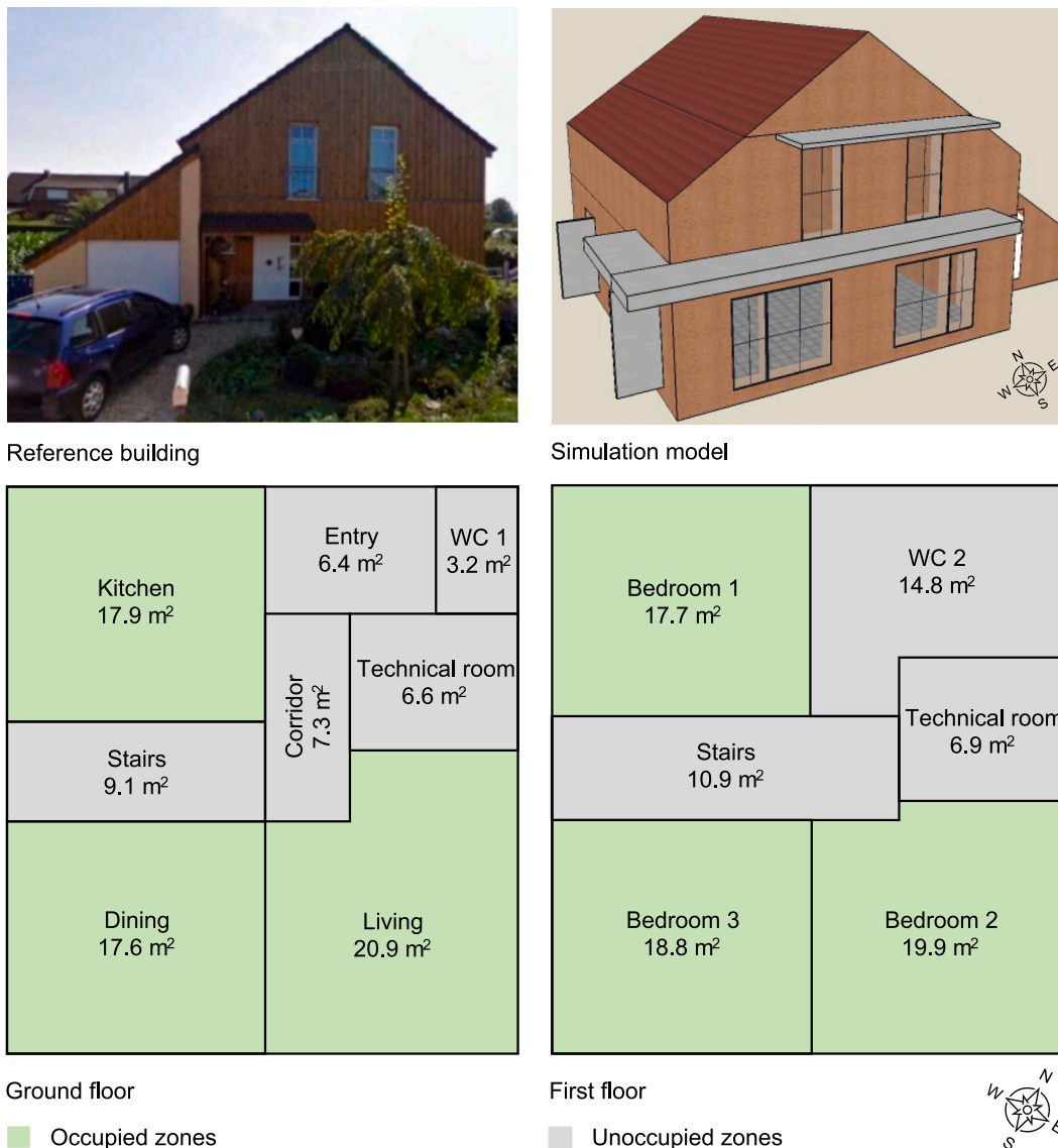
Fig. 3. Illustration of the real building, simulation model, and floor plans of the reference timber dwelling.
