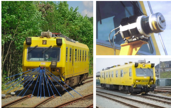
LiDAR data collection, EM130 vehicle Belgium
