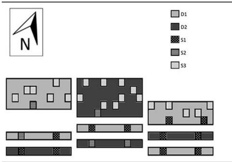
Figure 2-1 : Sun exposure and substrate depth modalities of the plots within the extensive plots of the TERRA building (Gembloux, Belgium). D1: shallow depth 6 cm - D2: deep depth 11 cm - S1: low sun exposure - S2: medium sun exposure - S3: high sun exposure
