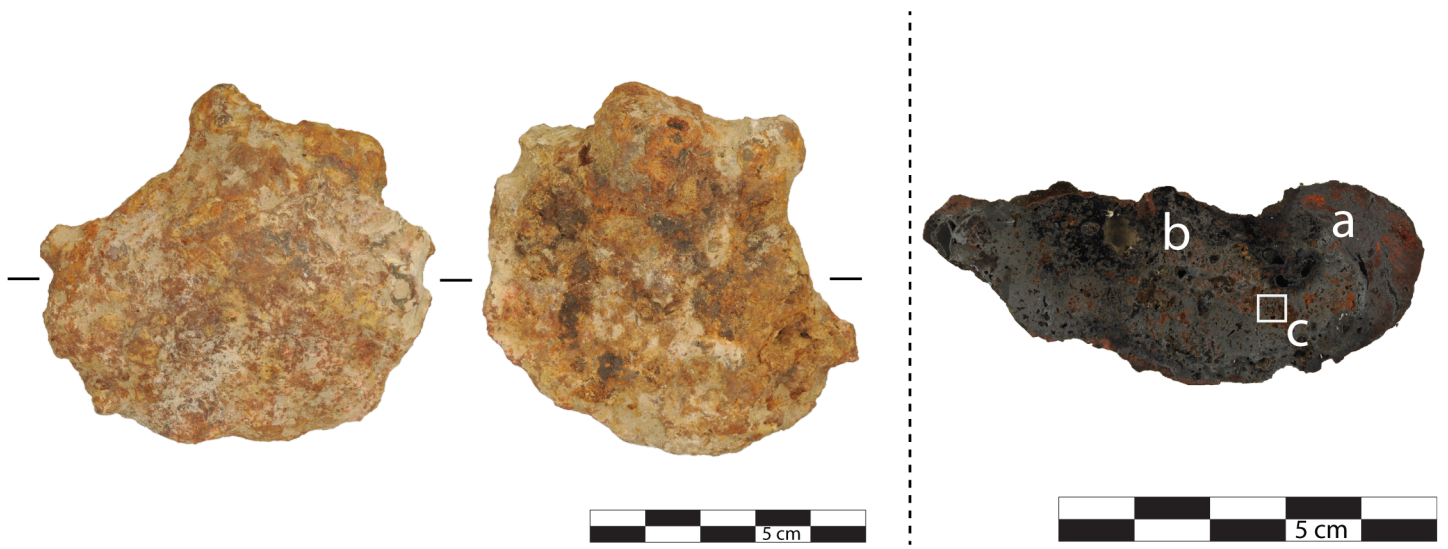
Small SFR hearth bottom. Mostly fayalite and dendritic wüstite (a). Many charcoal impressions (a, b) and corrosion product (c).
