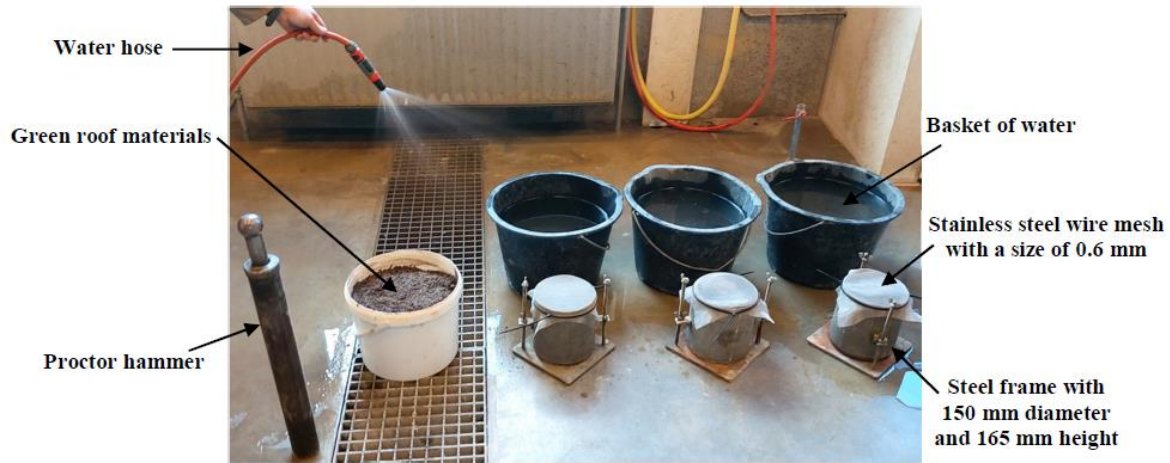
Fig. 2. 3. Apparatus used for the water retention capacity test.
