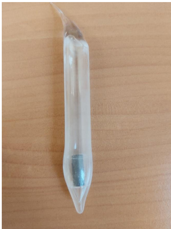
Figure 3-7: Closed evacuated silica tube with at its bottom the graphite crucible containing the sample.
