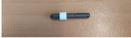
Figure B2: Glass cylinder fitting perfectly inside the alumina ring of the multi-anvil assembly.
