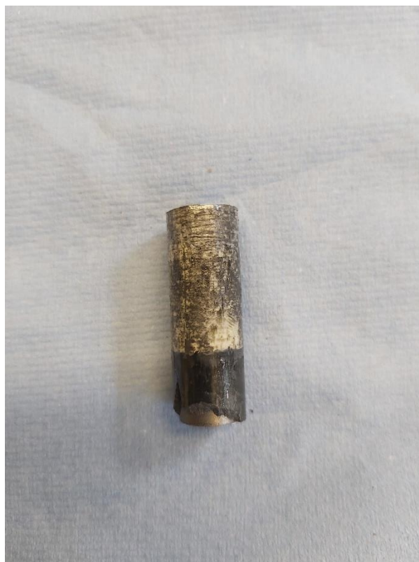
Figure 3-5: A BaCO 3 cell with the steel plug wrapped in pyrophyllite at the bottom after an experiment. BaCO 3 is very brittle, and so careful peeling is necessary to reach the capsule in the center without breaking it.
