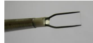
Total and static pressure, total temperature (AP1-C25 probe)
