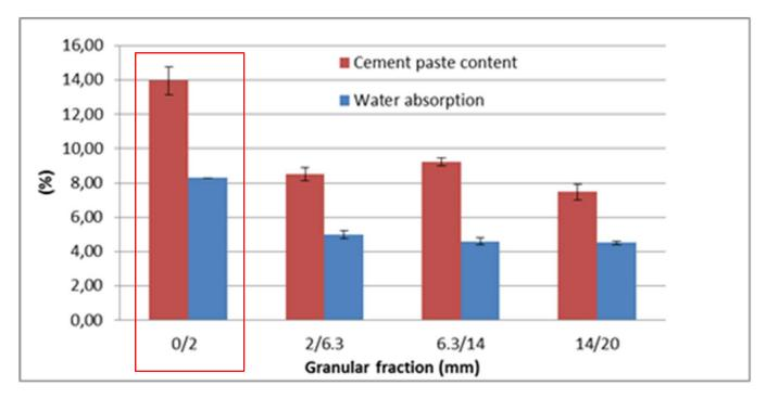
Cement Paste Content and W<sub>A</sub> of 0/2mm fraction larger than three coarse fractions
