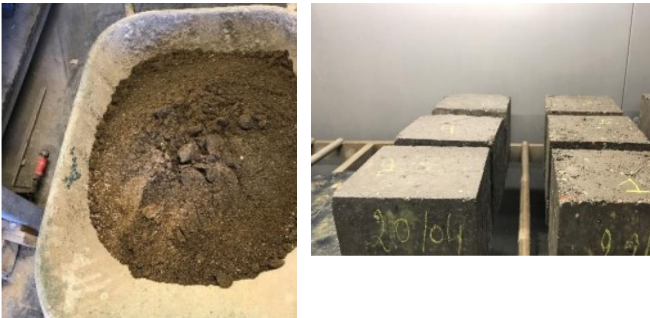
Figure 4: mix for rammed concrete and rammed concrete specimen [10]
