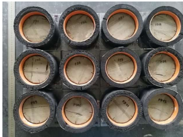
Figure 14: Visible spalling on the samples surface after 91 freeze-thaw cycles
