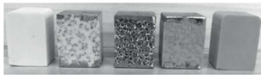
FIGURE 1.3: From right to left: silicon rubber specimen, silicon rubber/aluminum foam composite, aluminum foam only, room-temperature-vulcanising silicone/aluminum foam composite, room-temperature-vulcanising silicone only [186].
