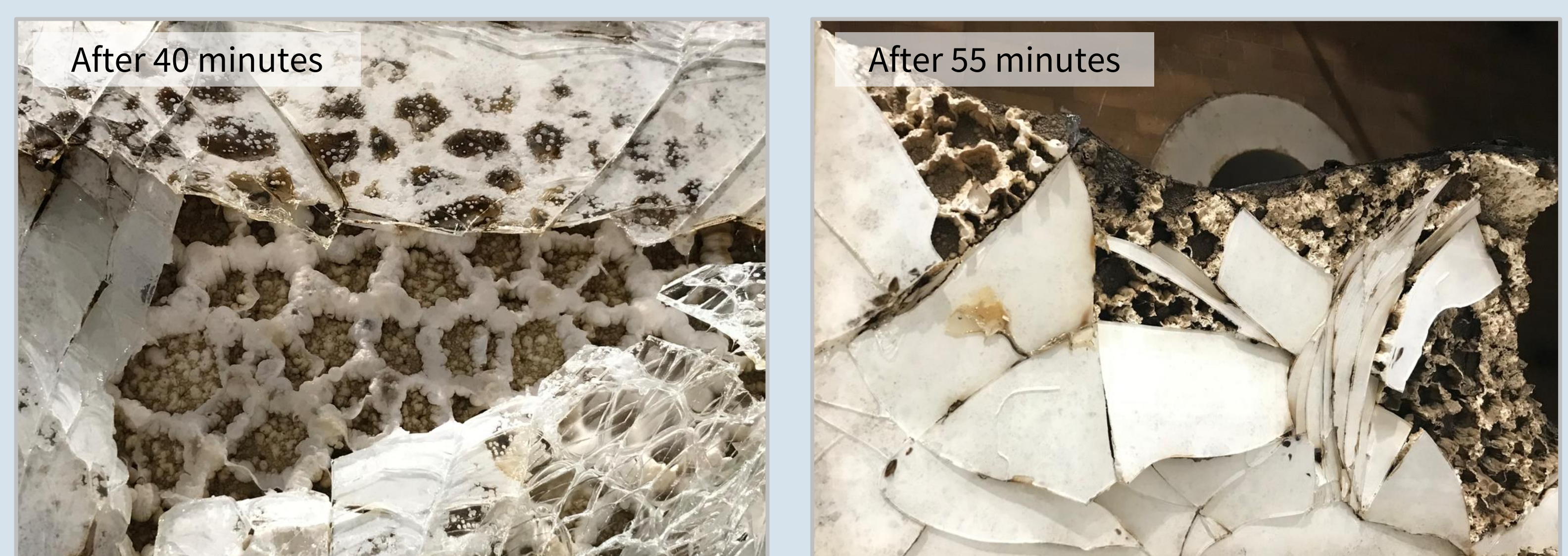
Fig. 5. Foam in the fire-resistant glass created in the full-scale fire test: after 40 and 55 minutes
