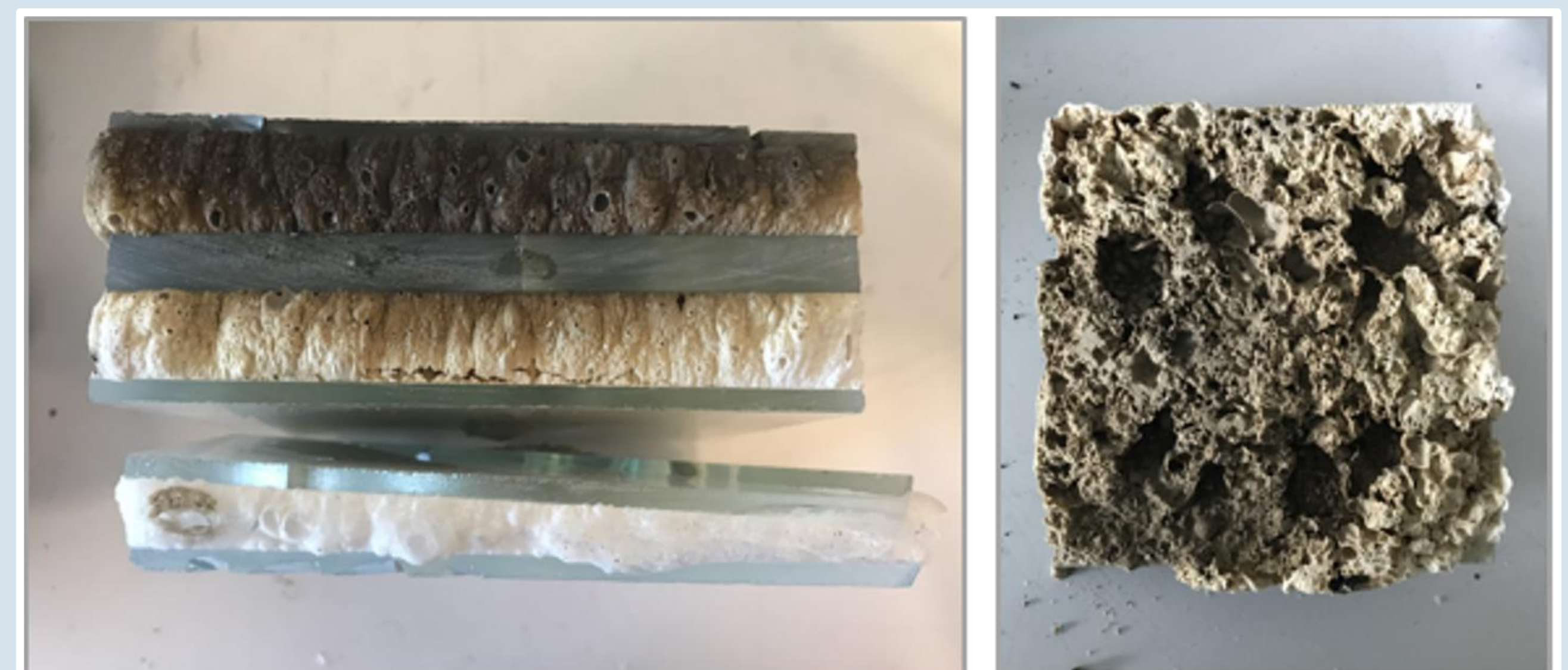
Fig. 2. Expanded fire-resistant glass and the created foam
