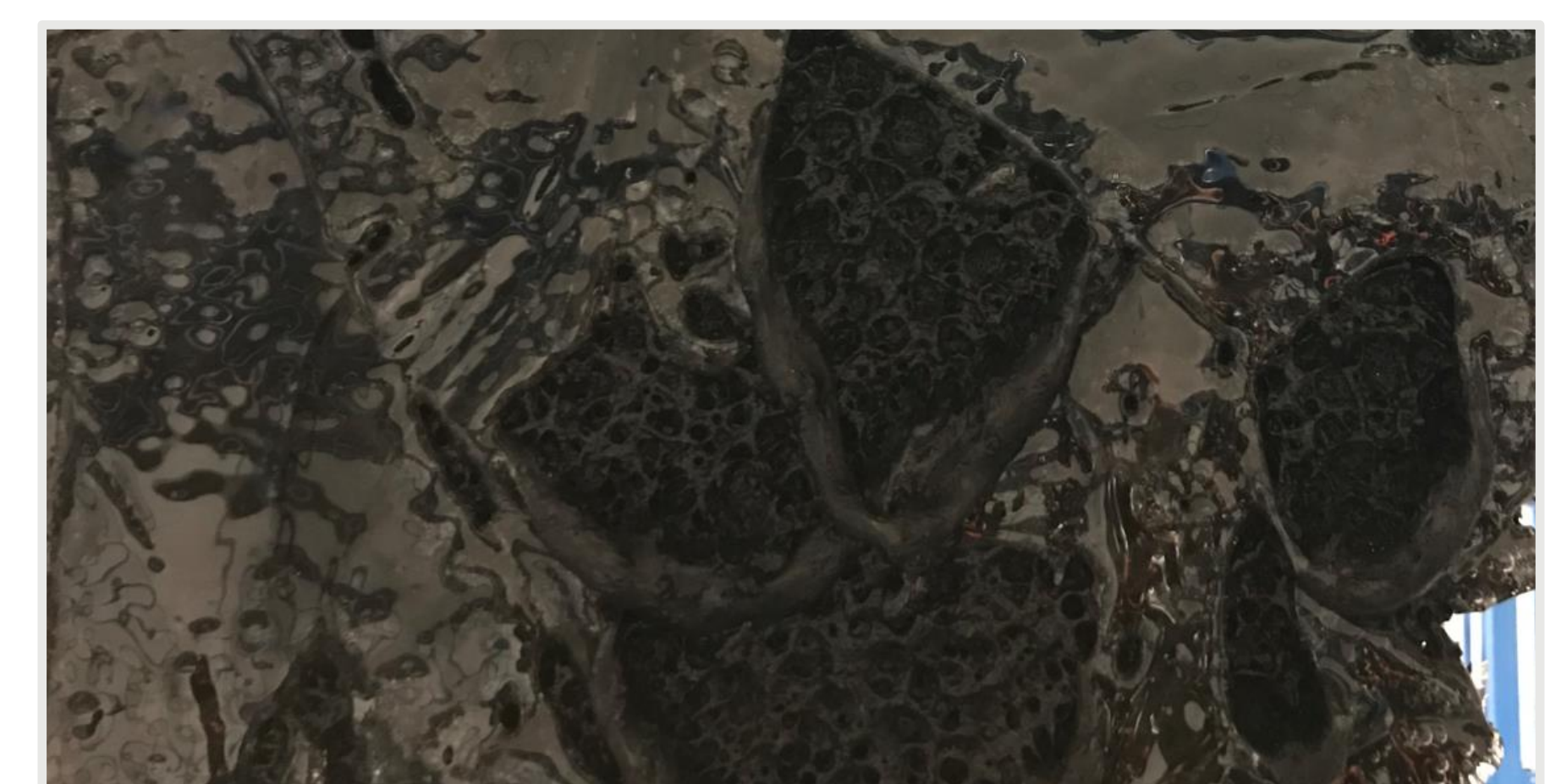
Fig. 4. Softening of the exposed glass and foam layers
