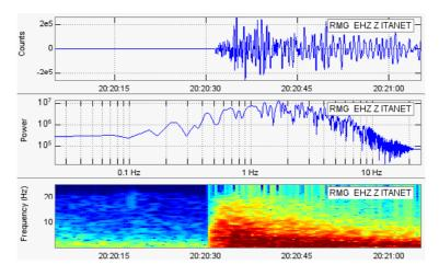
Fig. 7. Waveform, spectrogram and spectrum of a typical Hybrid event recored at Katale station renamed RMG after the deployement of the broadband 40s. the Frequency Contant reaches values about 8Hz.
