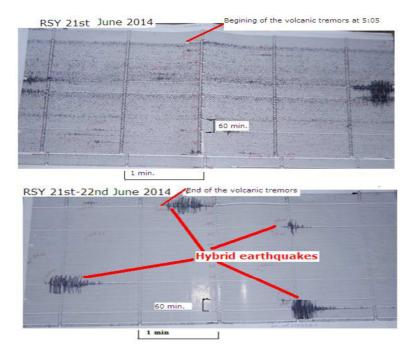
Figure 8: Typical seismograms recorded at Rusayo Analog station. Hybrid earthquakes and volcanic tremors are shown. The volcanic tremors began on 5:05 AM of 21st and finished on 17:04 of 21st by a hybrid earthquake
