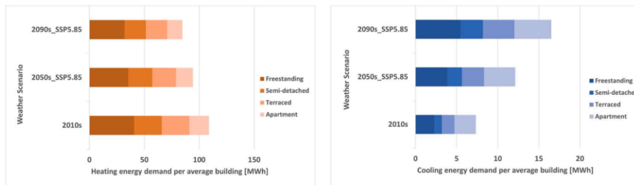
Fig. 15. Heating and cooling energy demands per average building type in the base scenario.
