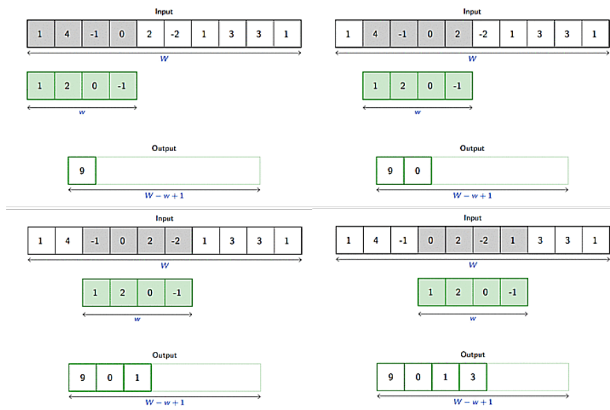
FIGURE 4.10: Illustration of how a convolution kernel is applied to a 1D array. From top left to bottom right, the kernel slides over the array, combining only the local information to produce an output value.
