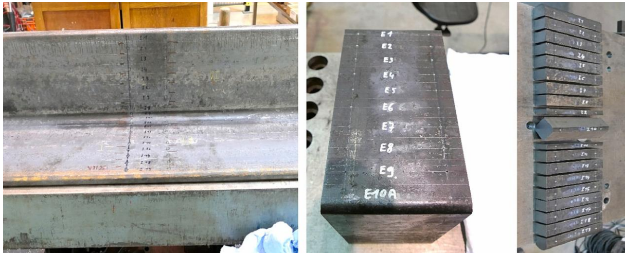
Fig. 10. Steps of the sectioning method for the tested profile: (a) mark of the specimens and reference points (left), (b) longitudinal sawing (middle), and (c) strip specimens (right).
