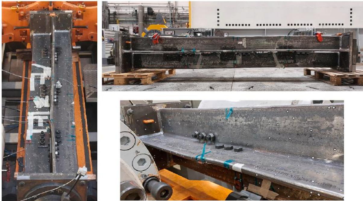
Fig. 22. Final deformation of the specimen.
