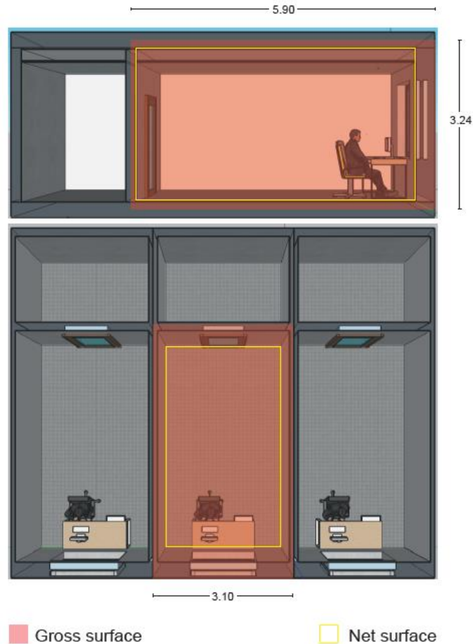
Figure 3.6 Definition of gross and net surface and volume and size of the office used in the model
