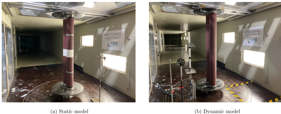
Figure 2. Experimental models in the test section: static (left), dynamic (right).
