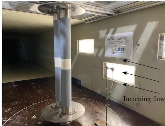
Figure 2. Experimental set-up installed in the wind tunnel of the University of Liège.
