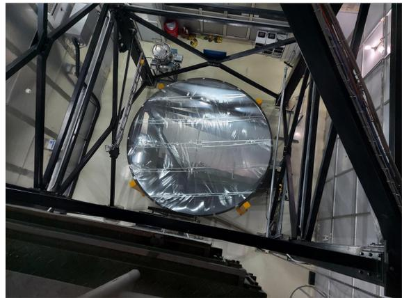
**Figure 6:** Top view of the ILMT mirror filled with mercury and covered with mylar
