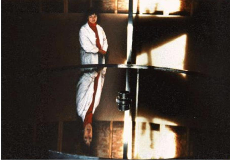
**Figure 1:** The UBC-Laval 2.7-m liquid mirror built in 1994.
