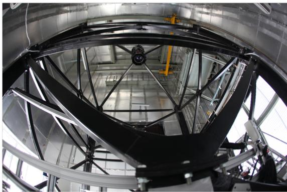
**Figure 5:** Fish eye view from bottom of the main ILMT structure and of the optical corrector at the very top.
