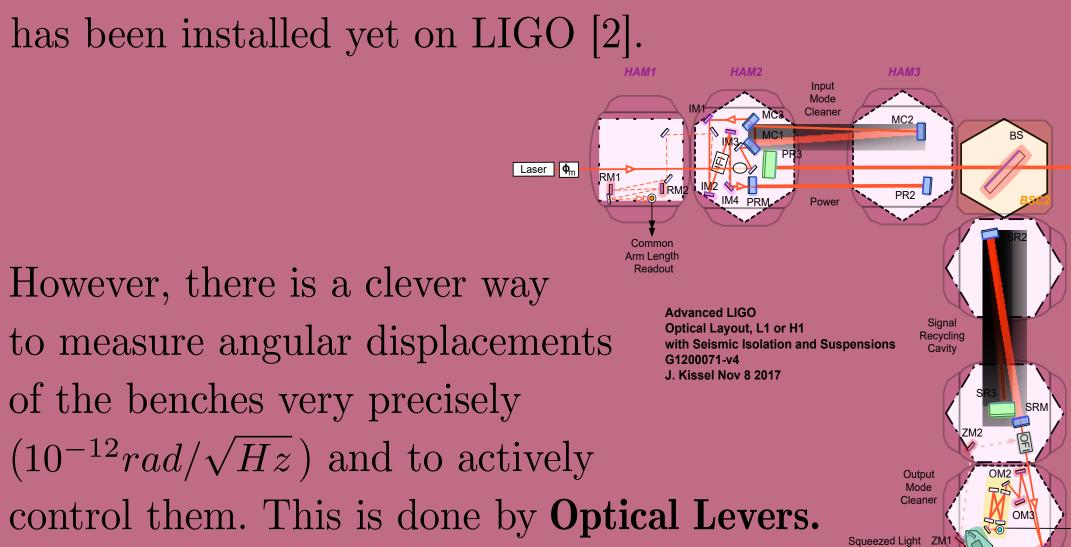
When the mirror is tilted, a spot displacement is recorded and the angle can be computed.
