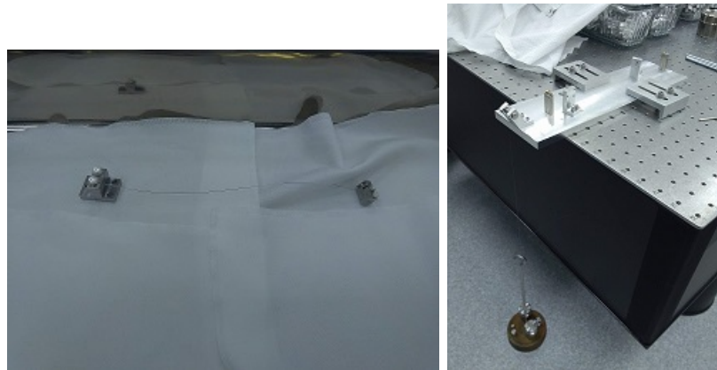
Figure A.2.: Left: one of the wire used to suspend the test mass. The wires suspending the bottom mass are stainless steel wires, 0.0047 inches-thick. The upper stages are suspended by 0.008 inches-thick wires. Right: Technique to prepare the wire with the right tension: a given weight is applied and left for 5 minutes.
