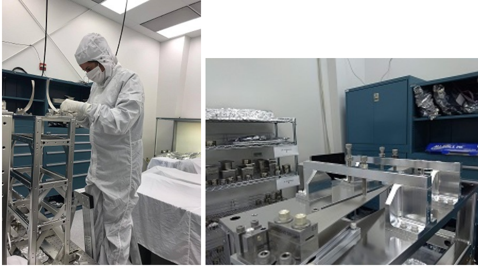
Figure A.1.: Mounting the blades onto the top of the suspension skeleton. On the right photo: the blades mounted and fixed and the required angle.
