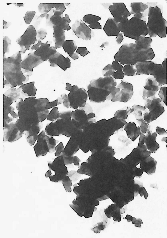
FIGURE 16 1. Well-crystallized hexagonal shaped particles of kaolinite from Brittany, France. X23 700 2. Kaolinite and mica flakes from a hydrothermally weathered granite in Brittany, France. X23 000 3. Kaolinite particles (below 1 micron) extracted from an altered granite (Cornwall, U.K.). X23 700 4. Well-crystallized kaolinite from tertiary sandy sediments in Southern Belgium. X30 000
