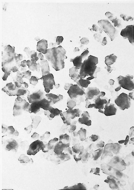
FIGURE 16 1. Well-crystallized hexagonal shaped particles of kaolinite from Brittany, France. X23 700 2. Kaolinite and mica flakes from a hydrothermally weathered granite in Brittany, France. X23 000 3. Kaolinite particles (below 1 micron) extracted from an altered granite (Cornwall, U.K.). X23 700 4. Well-crystallized kaolinite from tertiary sandy sediments in Southern Belgium. X30 000
