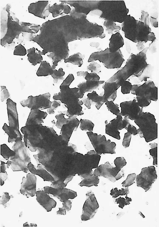
FIGURE 16 5. Partially b-axis disordered kaolinite particles from tertiary sands in Oret (Belgium) X30 000 6. Partially b-axis disordered kaolinite from tertiary residual clayey layers in Oret (Belgium) X30 000 7. Mixture of sericite (lathe-shaped particles) and badly crystallized kaolinite from tertiary weathered Cambrian arkosic quartzite in Ardennes, Belgium. X30 000 8. Mixture of badly crystallized kaolinite with some tubular forms (Germany) X23 700
