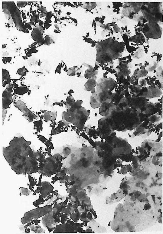
FIGURE 16 9. Kaolinite with muscovite particles from Germany X30 000 10. Tubular form (Halloysite from Utah (U.S.A.) X23 700 11. Tubular form (Halloysite) from Indiana (U.S.A.) X23 700 12. Illite and kaolinite, with goethite, from sandy layer in the residual tertiary cover of Southern Belgium. X30 000.
