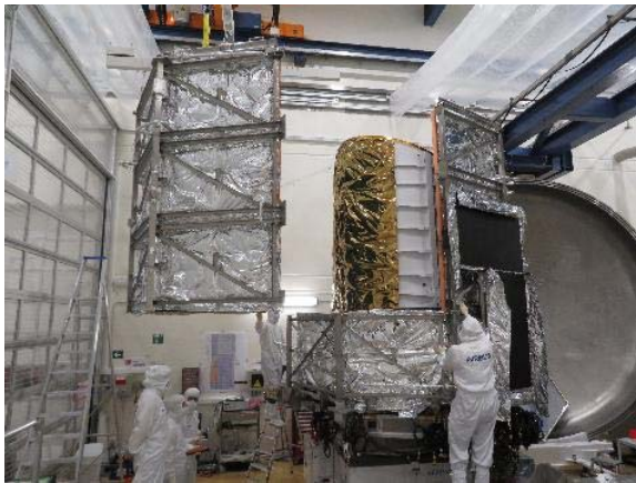
Picture 3-5: PLM Thermal Tent
