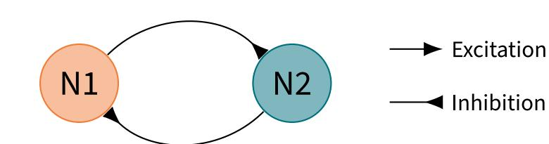
**Rebound bursting**: feature of biological neurons that our novel model brings to neuromorphic engineering. When a hyperpolarized (*i.e.* inhibited) neuron is dis-inhibited, it will fire a burst in the process of going back to its resting state. This feature allows robust, **self-sustaining oscillations** of the half-center oscillator.
