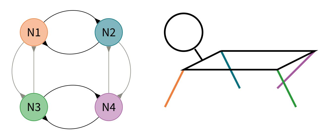
Each neuron of a CPG can be **individually neuromodulated** to produce **different locomotion pat-terns** while preserving the robust global rhythm of the system.
