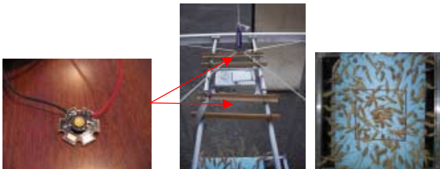
Figure 5. The Power-leds used (left); their location (middle); one image took with the two Leds (right).
