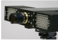
Figure 2. A 3D camera (by PMD Technologies). Two arrays of infrared LEDs are located on both sides of the sensor.
