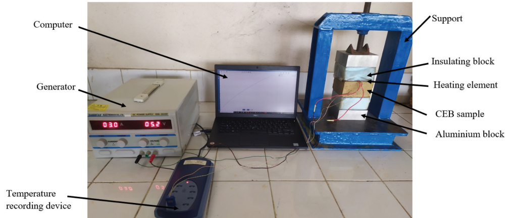
Figure 13. Experimental asymmetric hot plate device.
