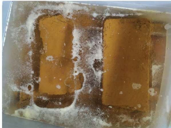
Figure 23. Unstabilized CEB destroyed during water absorption test.
