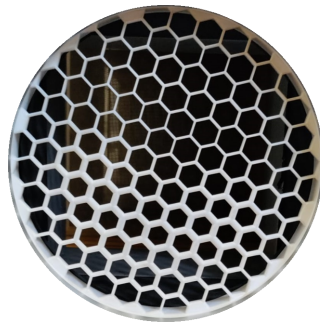
Figure 1: A total pressure distortion generator
