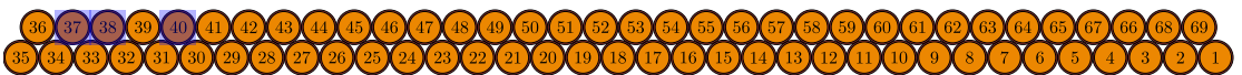
FIGURE 3.10: The turns of the 69 turns winding on which the time domain experimental investigation is performed are highlighted in blue.
