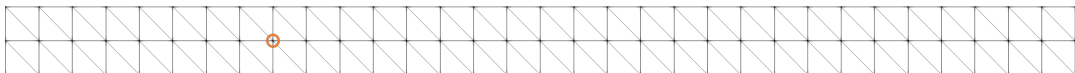
FIGURE 3.23: Mesh with 33x3 nodes and 128 elements. The temperature is extracted at the marked node at x = 1 m and y = 0.125 m.
