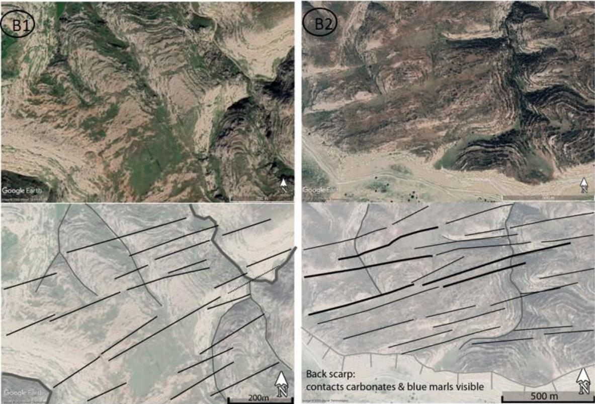
**Figure 3.7.** A. Google Earth Image showing the fracture network parallel to the Relizane Fault. B. Details of the fracture network mapped using very high-resolution satellite images from Google Earth.
