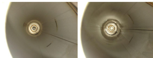
Fig. 3 Inside of the UVozone reactor before (left) and after (right) deposition of the aqueous TiO 2 coating
