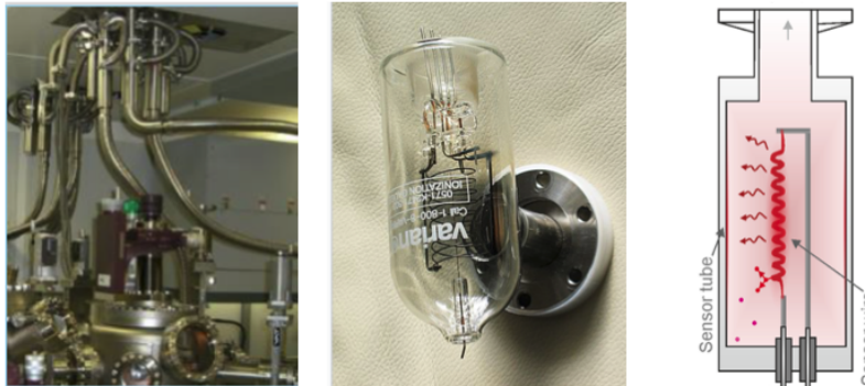
Figure 3.8: Pictures of a liquid nitrogen feed lines coming from a phase separator (left), an ion gauge (middle) and a Pirani gauge filaments (right).
