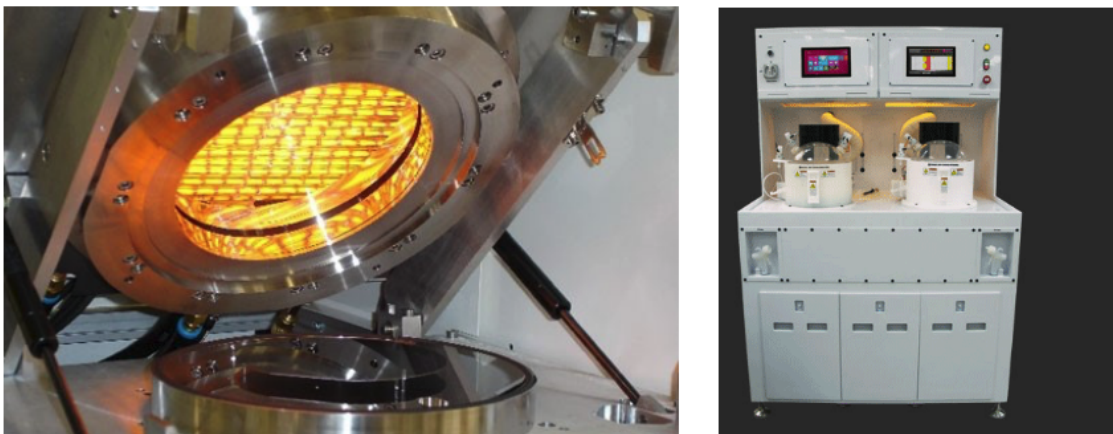
Figure 3.14: A rapid thermal annealing chamber with heating lamps (left) and a wet processing unit to clean wafers (right).
