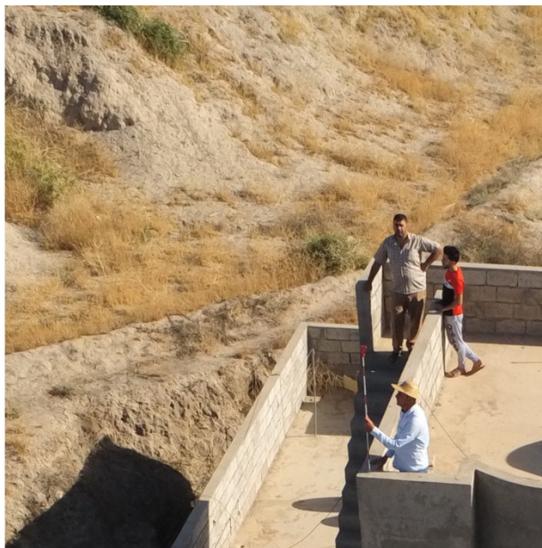
FIG. 2: Illustration of topographic ground measurements, one of the ground targets (left) and Omar Sharef operating the total station prism at a roof corner of a modern building (MAA)
