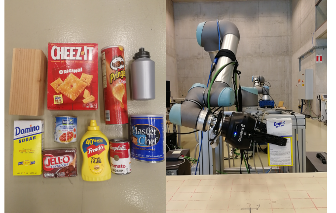
Fig. 4: (left) Object assets used in the real setup. (right) Example of side grasp.
