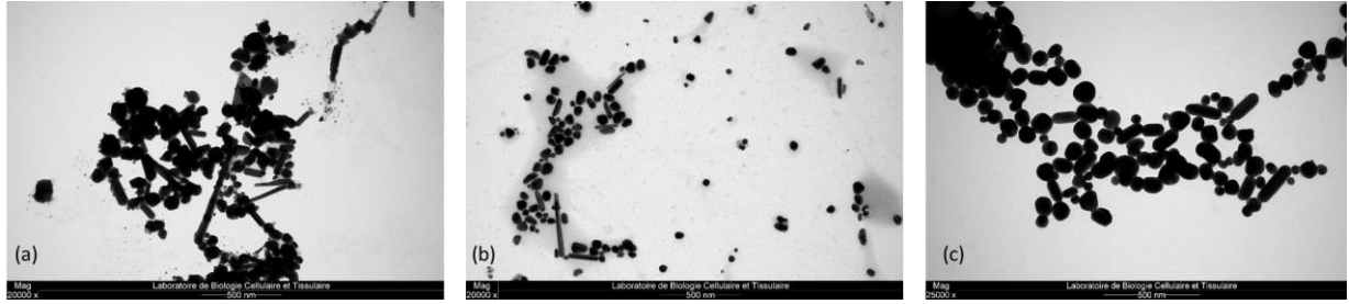
Figure 6: Transmission electron microscopy (TEM) pictures with a 20 000 magnification of silver nanoparticles synthesized by chemical reduction during the early characterization design. Several syntheses were observed with different polydispersity index (PDI), (a) Synthesis 7A with a PDI of 0.422; (b) Synthesis 2B with a PDI 0.322; (c) Synthesis 12A with a PDI of 0.181.
