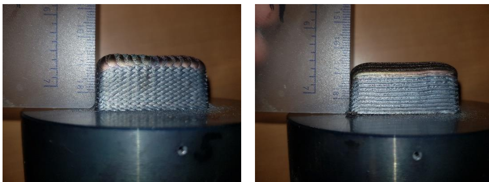
Fig. S.1: Both sides of LFP1 sample in the as-built conditions, with no visible cracks within the As built deposit.
