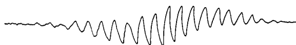
FIG. 1. Derivative of resonance absorption ( dX''/dH ) vs field ( H ) of a dilute solution of anthracene in sulfuric acid.
