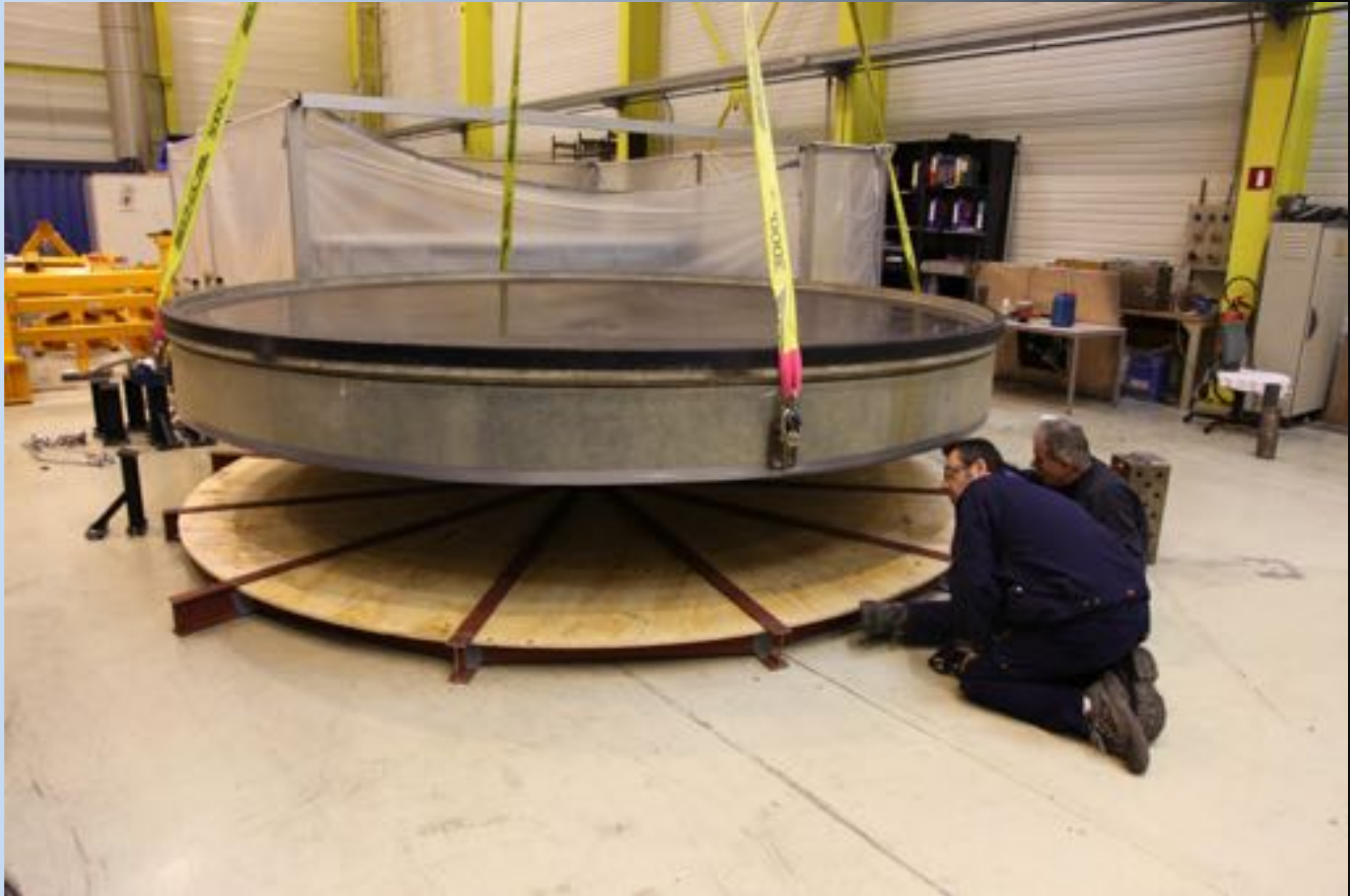
Packing of the mirror with foam, carbon fiber and polyurethane at AMOS, before shipping from Liège to ARIES observatory (Devasthal, India) on the 22nd of December 2011.
