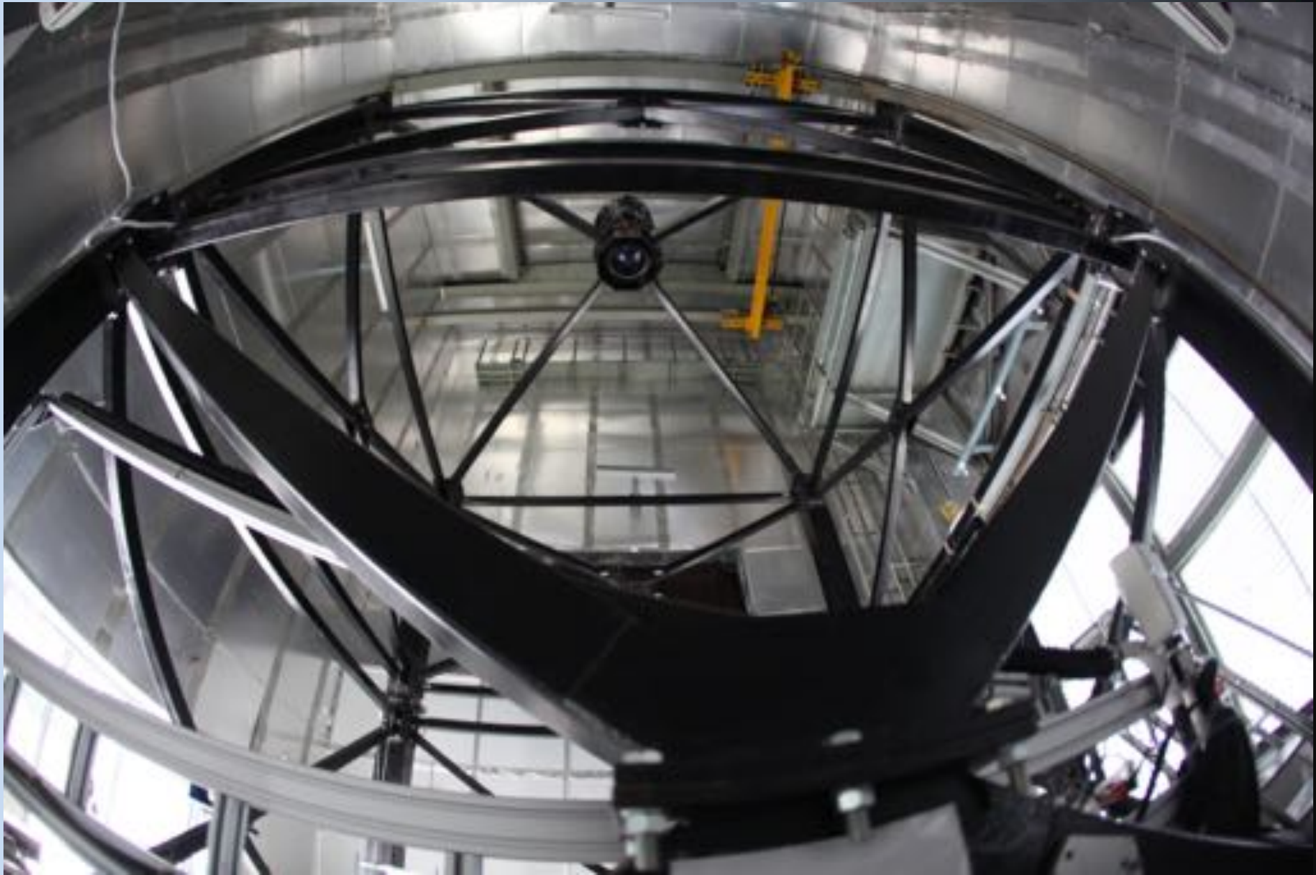
Fish eye view of the main ILMT structure and of the optical corrector.
