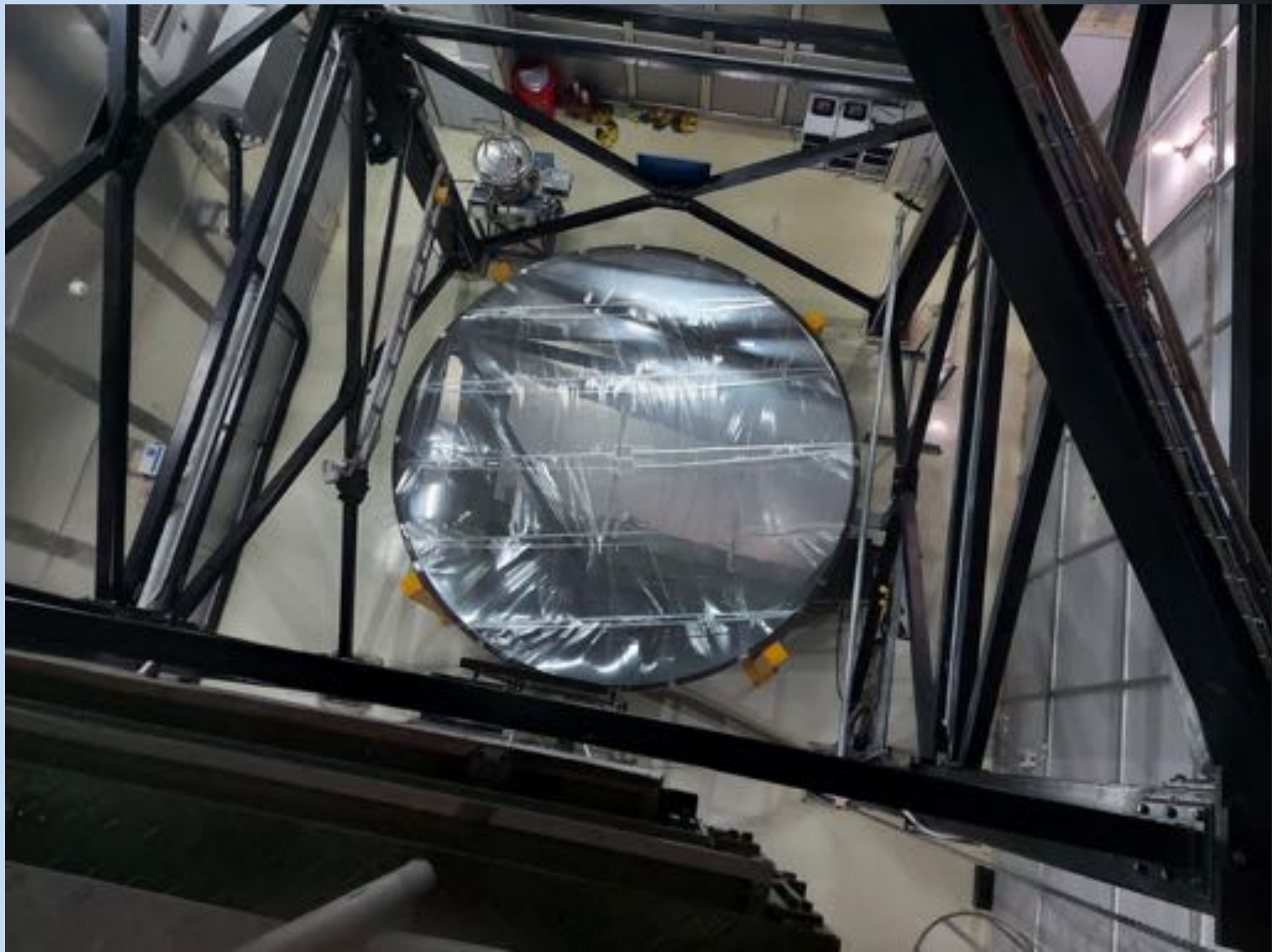
The ILMT mirror filled with mercury and covered with mylar
