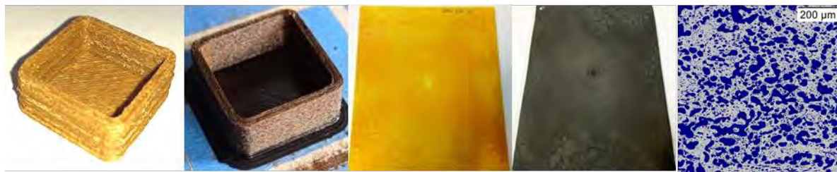
FIGURE 1: 3D-printed cups, novolac-based (left), lignin-based (middle-left), injection moulded plate (middle), corresponding porous carbon plate (middle-right), micrograph of porous carbons (white: carbon, right).
