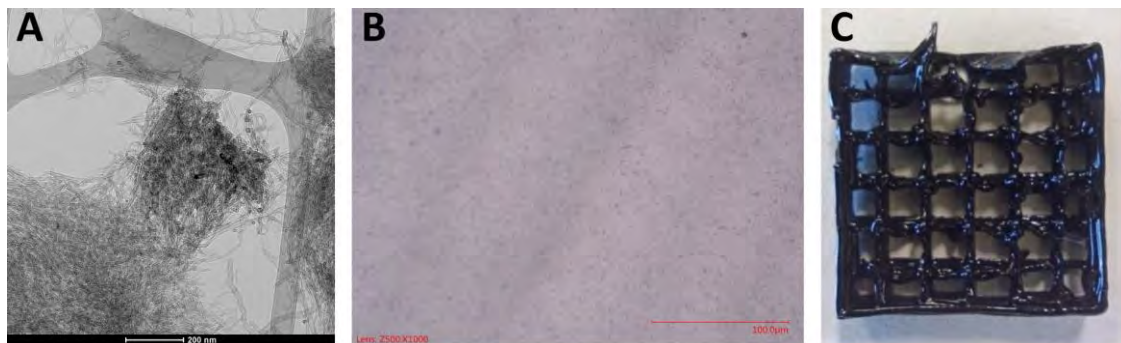
FIGURE 1: TEM image of MWCNTs which shows the tendency of nanomaterial to form agglomerate structures (A); image from the optical microscope that presents overall MWCNTs distribution in composite's volume (B); the photo of composite 3D printed with the use of CellInk BioX device (C).
