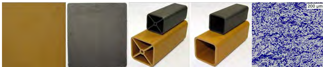
FIGURE 2: pressed board (left), corresponding porous carbon (middle-left), extruded NFC profiles with corresponding porous carbons (middle, middle-right), micrograph of porous carbons (white: carbon, right).
