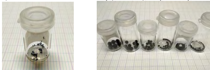
FIGURE 3: Hollow carbon spheres: of the same diameter (0.8 - 1 mm) and different conductivities (from 3.5 \times 10^{-6} to 15 \times 10^3 S/m) on the one hand (left), and of different diameters (5, 4, 3, 2, 1 and 0.8 mm) but the same conductivity (125 S/m) on the other hand (right).
