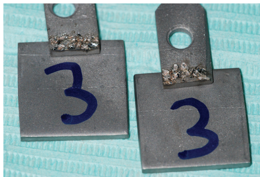
FIGURE 4: Plates of group C soldered by the electrowelder.
