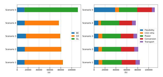
**Figure 3**: (a): Breakdown of costs per scenario and per cluster (Belgium (BE), Algeria (DZ), and Greenland (GL)). (b): Breakdown of costs per scenario per asset function. Flexibility covers storage capacities, CO2 Infra covers CO2 capture, storage, and transport, Power covers means of electricity production, Conversion covers all assets that convert one commodity into another and Transport HVDC lines and CH4 carriers.
