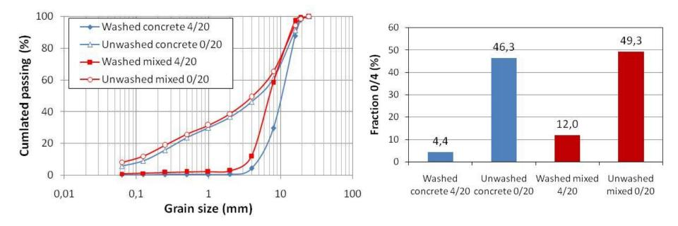
Fine content (< 63µm) higher in mixed aggregates and significantly reduced by washing
