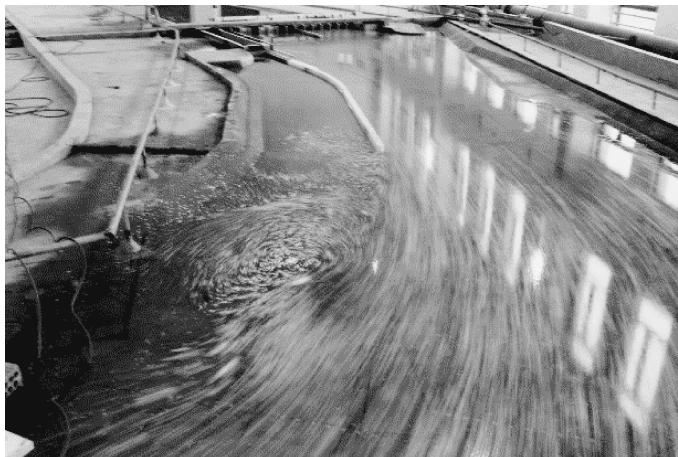
Fig. 3. Flow regime in downstream entrance area for Q=1,008 \text{ m}^3/\text{s} .
