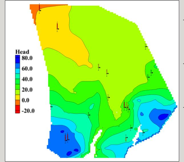
$\rightarrow$  The transient model the period covers between 1990 and 2020  $\rightarrow$  It integrates the temporal variation of the recharge and the pumping rates  $\rightarrow$  It was calibrated using the piezometric heads in each aquifer
