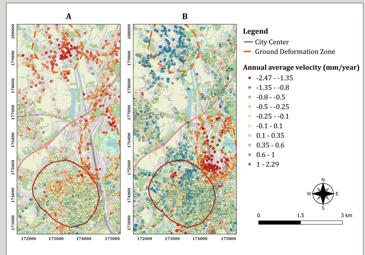
$\rightarrow$  Identification of the two ground deformation zones located North of Leuven using InSAR data from the ERS1/2 (A) and
