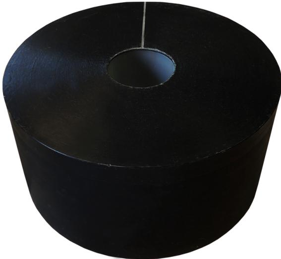
FIGURE 5.2: Picture of the Halbach cylindrical magnet used.
