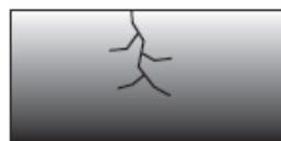
Stress corrosion cracking
