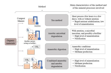
**Figure 1.** Summary diagram of tea, aerobic microbial degradation, anaerobic digestion and combined anaerobic–aerobic degradation methods for the production of organic nutrient solution.
