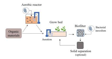
**Figure 2.** Schematic of organic materials aerobic degradation integrated and/or external to the bioponic system.
