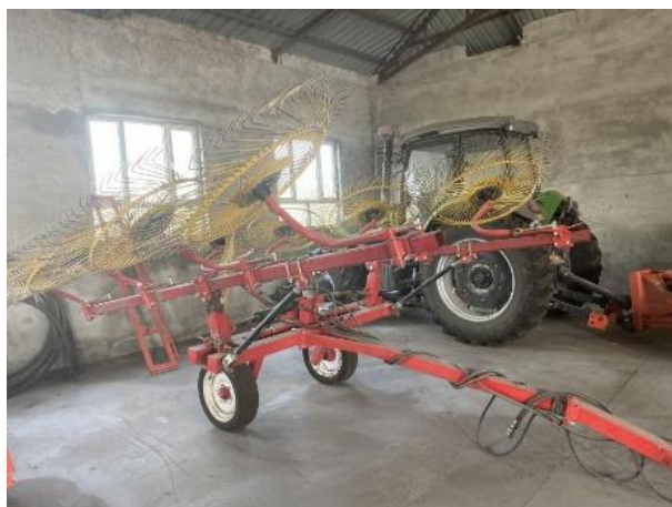
Figure 5-1: Example of a typical hayrake used in Jilin province (Photograph taken by the author of thesis)
