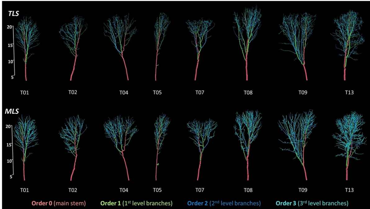
Figure 43. Examples of the quantitative structural models (QSMs) of hardwood trees reconstructed from TLS (top) and MLS (bottom) point clouds. Colors represent branching orders: red (order 0 - main stem), green (1st-order branches), blue (2nd-order branches), cyan (3rd-order branches).
